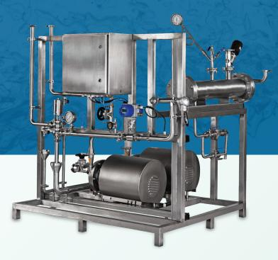
WFI is collected in SS 316L storage tank and is circulated across the user points at 75 to 80 Deg C temperature with help of process loop pumps. The loop return velocity is maintained by synchronising the Flow Transmitter and loop pumps with VFD through PLC. Loop is sanitized by heat exchangers in the return line or steam jacketed WFI tank.
